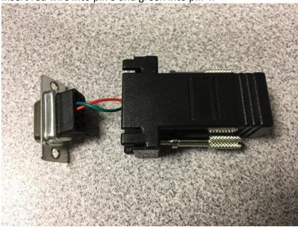
Trim off connectors from unused wires to avoid shorts. Tuck unused wires into adapter housing and snap connector back in place:
